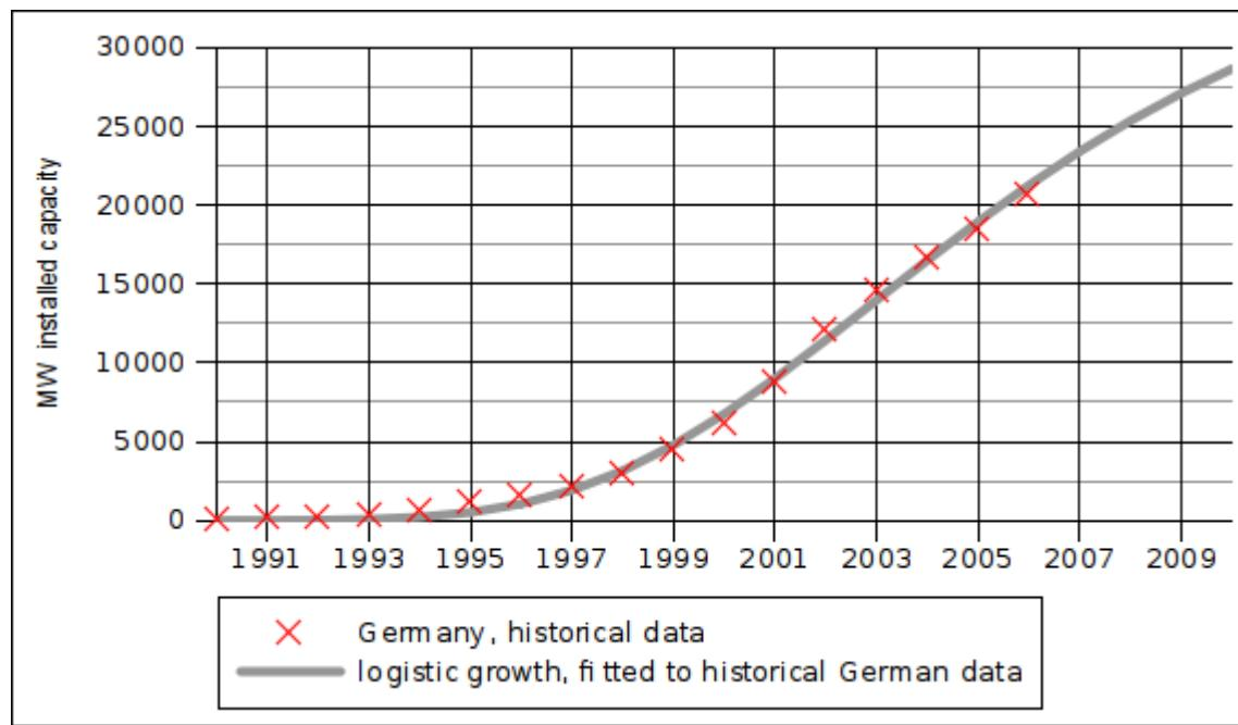
Figure 8: Example for fitting the logistic growth function used in the "REO 2030" scenarios to historical data of Wind Energy development in Germany.
