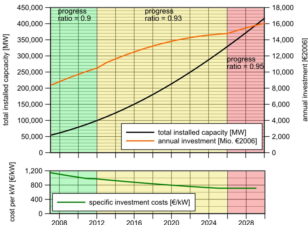
Figure 9: Example for calculating technology cost decrease by progress ratio. [EWG; 2008]
