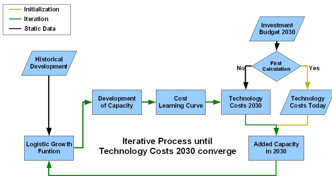
Figure 5: Flow chart of the scenario development process with iteration of technology costs and added capacities in 2030. [S. Peter, H. Lehmann; 2007]
