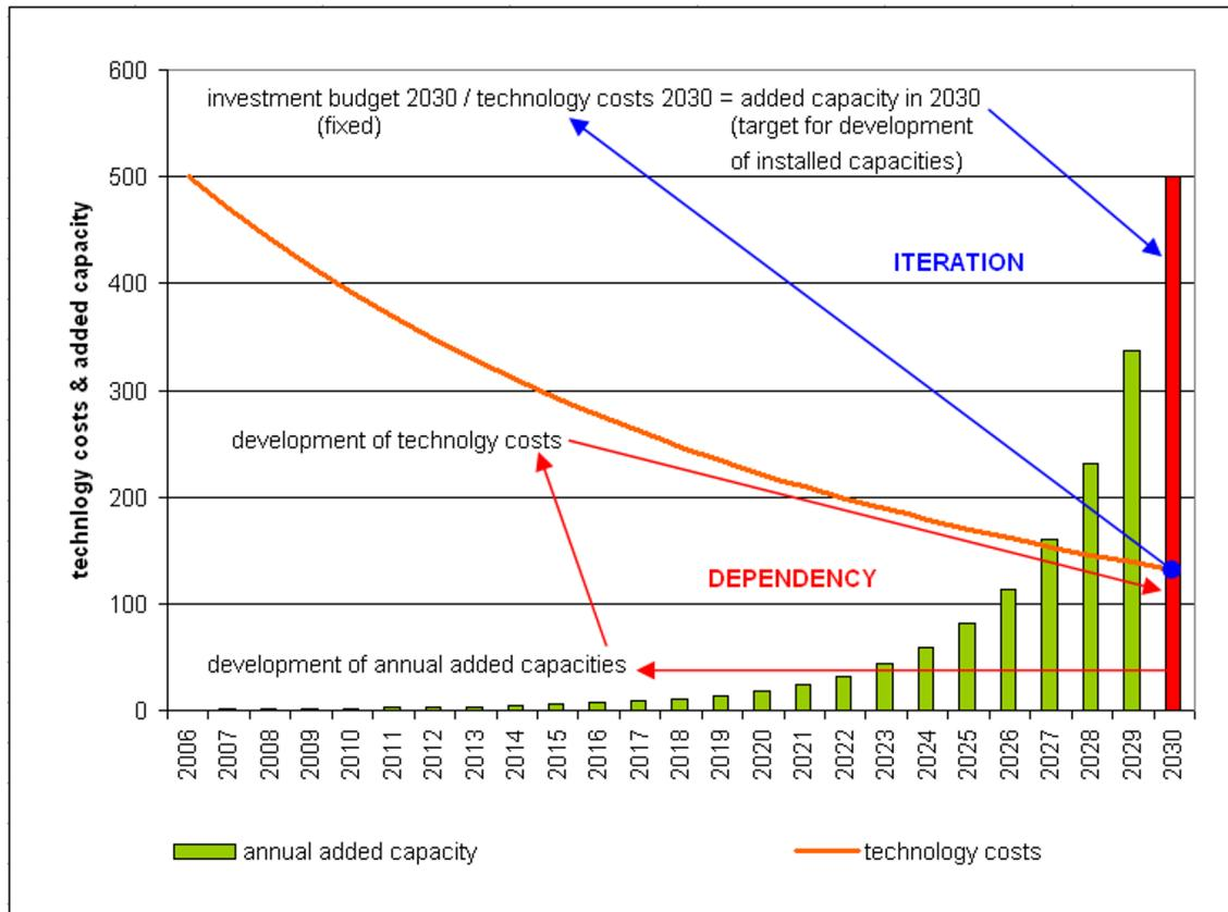
Figure 6: Example of translating the 2030 investment budget into new added capacities in 2030 with regard to degression of specific technology costs (see also Figure 5 on page 19 for more information on iterative technology cost calculation). [S. Peter, H. Lehmann; 2007]
